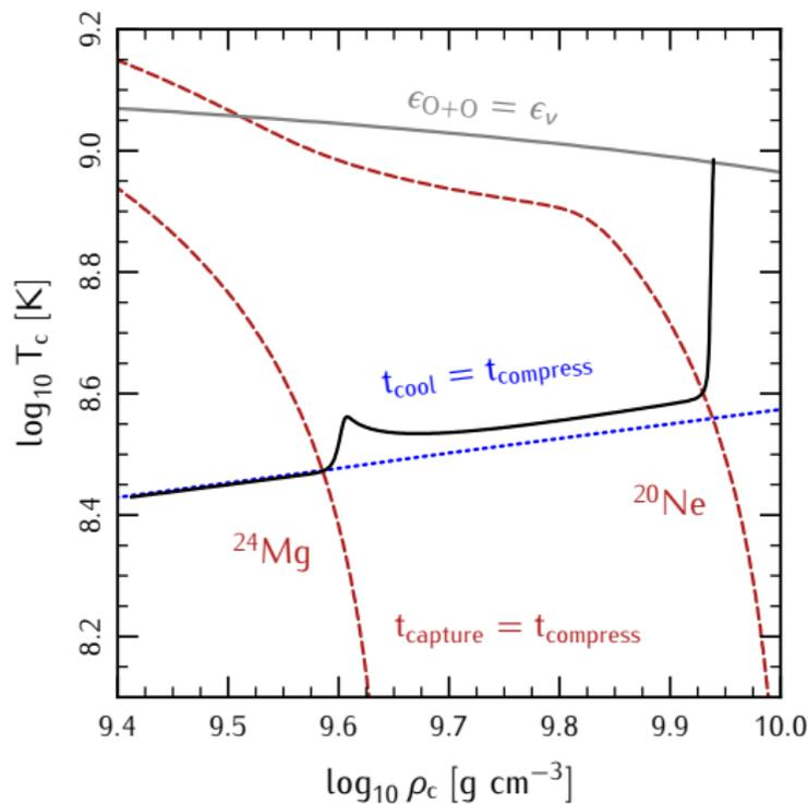
A thermal runaway develops in the core;
